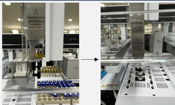
Fig. 4f Drawing sample and subsequent injection into GCMS using the a 10-µL syringe.
