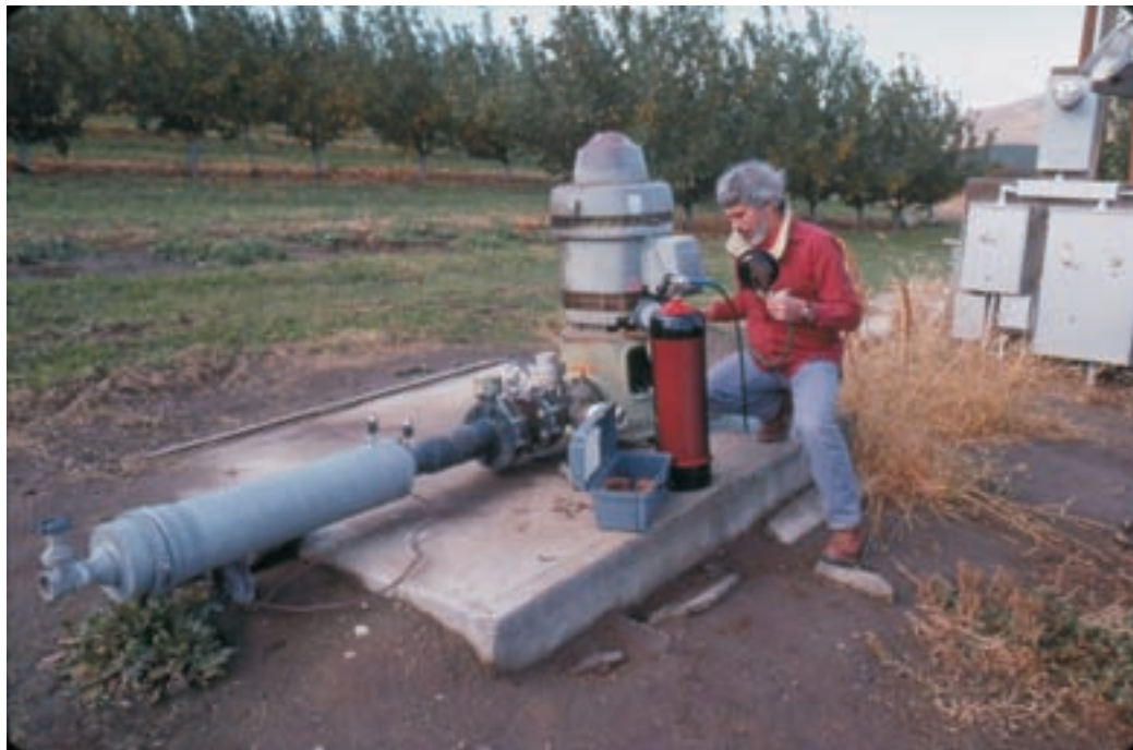
Ecology's Robert Garrigues, measuring the static water level of an irrigation well in the Yakima River Watershed.
