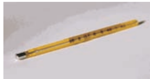
Mercury, a metal which is a Persistent Bioaccumulative Toxin, is used in fever thermometers, which are now being replaced by safer digital thermometers.
