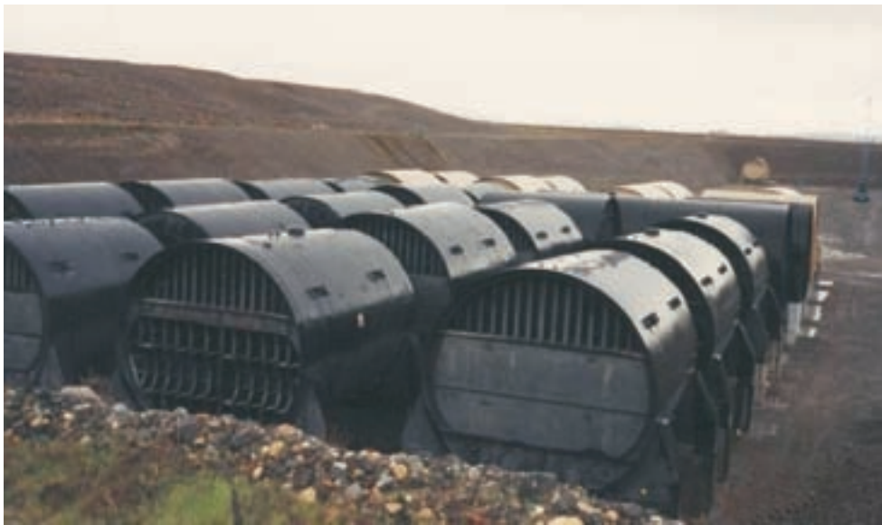
Submarine nuclear reactor core vessels in a Hanford Nuclear Reservation disposal trench.
