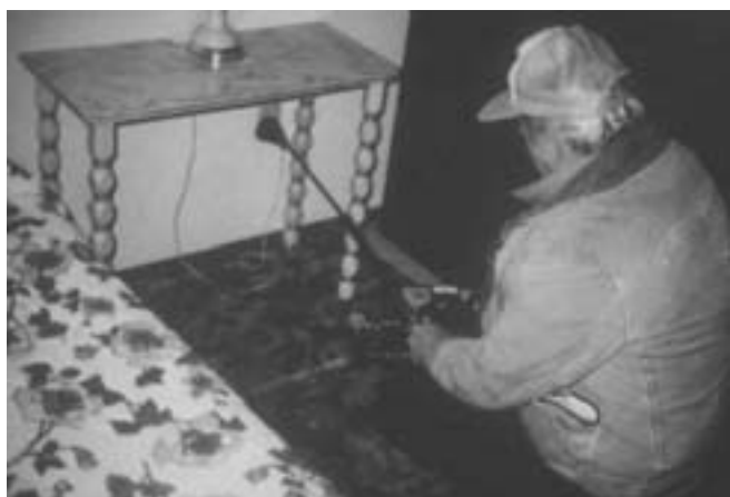
Sampling for combustible gases in a Midway area home, 1985
